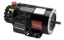
Marathon Black MAX high efficiency AC induction motor, highperformance inverter duty, 7-1/2hp, 3-phase, 230/460 VAC, 1800rpm, TENV, NEMA 213TC frame, cast aluminum, C-face/rigid base mount. Dynapar HS35 encoder included.
