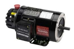
Marathon Black MAX high efficiency AC induction motor, high-performance inverter duty, 7-1/2hp, 3-phase, 230/460 VAC, 1800rpm, TENV, 213TC frame, cast aluminum, C-face/rigid base mount. Dynapar HS35 encoder included.
