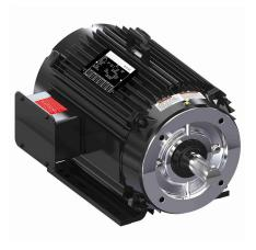
Marathon Black MAX standard efficiency AC induction motor, high-performance inverter duty, 5hp, 3-phase, 230/460 VAC, 1200rpm, TENV, NEMA 215TC frame, cast aluminum, C-face/rigid base mount.
