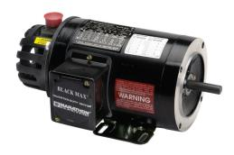
Marathon Black MAX standard efficiency AC induction motor, high-performance inverter duty, 5hp, 3-phase, 230/460 VAC, 1200rpm, TENV, NEMA 215TC frame, cast aluminum, C-face/rigid base mount. Dynapar HS35 encoder included.
