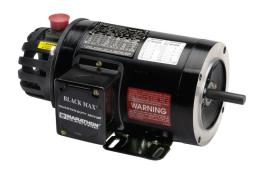
Marathon Black MAX premium efficiency AC induction motor, high-performance inverter duty, 5hp, 3-phase, 230/460 VAC, 1800rpm, TENV, NEMA 184TC frame, aluminum, C-face/rigid base mount. Dynapar HS35 encoder included.
