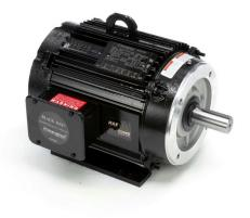
Marathon Black MAX standard efficiency AC induction motor, high-performance inverter duty, 3hp, 3-phase, 230/460 VAC, 1200rpm, TENV, NEMA 213TC frame, cast aluminum, C-face/rigid base mount.
