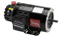
Marathon Black MAX standard efficiency AC induction motor, high-performance inverter duty, 3hp, 3-phase, 230/460 VAC, 1200rpm, TENV, NEMA 213TC frame, cast aluminum, C-face/rigid base mount. Dynapar HS35 encoder included.
