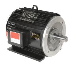
Marathon Black MAX high efficiency AC induction motor, high-performance inverter duty, 3hp, 3-phase, 230/460 VAC, 1800rpm, TENV, 182TC frame, aluminum, C-face/rigid base mount.
