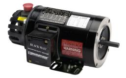
Marathon Black MAX high efficiency AC induction motor, highperformance inverter duty, 3hp, 3-phase, 230/460 VAC, 1800rpm, TENV, NEMA 182TC frame, aluminum, C-face/rigid base mount. Dynapar HS35 encoder included.
