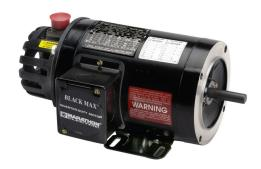
Marathon Black MAX high efficiency AC induction motor, high-performance inverter duty, 3hp, 3-phase, 230/460 VAC, 1800rpm, TENV, 182TC frame, aluminum, C-face/rigid base mount. Dynapar HS35 encoder included.
