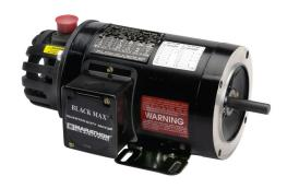
Marathon Black MAX standard efficiency AC induction motor, high-performance inverter duty, 2hp, 3-phase, 230/460 VAC, 1200rpm, TENV, NEMA 184TC frame, cast aluminum, C-face/rigid base mount. Dynapar HS35 encoder included.
