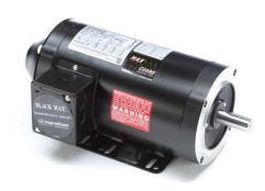
Marathon Black MAX high efficiency AC induction motor, high-performance inverter duty, 1-1/2hp, 3-phase, 230/460 VAC, 1800rpm, TENV, NEMA 145TC frame, rolled steel, C-face/rigid base mount.
