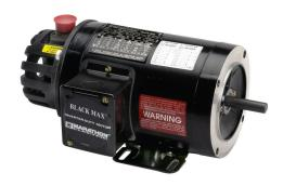
Marathon Black MAX high efficiency AC induction motor, high-performance inverter duty, 1-1/2hp, 3-phase, 230/460 VAC, 1800rpm, TENV, NEMA 145TC frame, rolled steel, C-face/rigid base mount. Dynapar HS35 encoder included.
