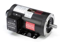
Marathon Black MAX high efficiency AC induction motor, high-performance inverter duty, 1hp, 3-phase, 230/460 VAC, 1200rpm, TENV, 145TC frame, rolled steel, C-face/removable rigid base mount.
