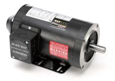
Marathon Black MAX high efficiency AC induction motor, highperformance inverter duty, 1hp, 3-phase, 230/460 VAC, 1800rpm, TENV, NEMA 143TC frame, rolled steel, C-face/removable rigid base mount.
