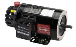
Marathon Black MAX high efficiency AC induction motor, highperformance inverter duty, 1hp, 3-phase, 230/460 VAC, 1800rpm, TENV, NEMA 143TC frame, rolled steel, C-face/removable rigid base mount. Dynapar HS35 encoder included.
