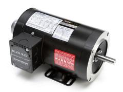
Marathon Black MAX high efficiency AC induction motor, high-performance inverter duty, 1hp, 3-phase, 230/460 VAC, 1800rpm, TENV, 56C frame, rolled steel, C-face/removable rigid base mount.
