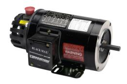
Marathon Black MAX high efficiency AC induction motor, high-performance inverter duty, 1hp, 3-phase, 230/460 VAC, 1800rpm, TENV, 56C frame, rolled steel, C-face/removable rigid base mount. Dynapar HS35 encoder included.
