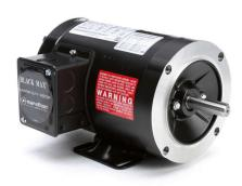
Marathon Black MAX premium efficiency AC induction motor, high-performance inverter duty, 1/2hp, 3-phase, 230/460 VAC, 1800rpm, TENV, NEMA 56C frame, rolled steel, C-face/removable rigid base mount.
