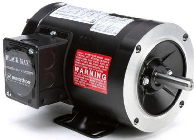
Marathon Black MAX premium efficiency AC induction motor, high-performance inverter duty, 1/2hp, 3-phase, 230/460 VAC, 1800rpm, TENV, NEMA 56C frame, rolled steel, C-face/removable rigid base mount.
