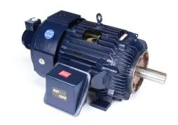
Marathon Blue MAX high efficiency AC induction motor, highperformance inverter duty, 100hp, 3-phase, 230/460 VAC, 1800rpm, TEBC, 405TC frame, cast iron, C-face/rigid base mount.
