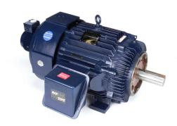
Marathon Blue MAX high efficiency AC induction motor, high-performance inverter duty, 100hp, 3-phase, 230/460 VAC, 1800rpm, TEBC, NEMA 405TC frame, cast iron, C-face/rigid base mount.
