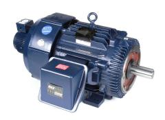
Marathon Blue MAX standard efficiency AC induction motor, high-performance inverter duty, 75hp, 3-phase, 230/460 VAC, 1800rpm, TEBC, NEMA 365TC frame, cast iron, C-face/rigid base mount.
