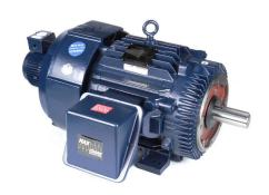
Marathon Blue MAX standard efficiency AC induction motor, high-performance inverter duty, 75hp, 3-phase, 230/460 VAC, 1800rpm, TEBC, NEMA 365TC frame, cast iron, C-face/rigid base mount. Dynapar HSD38 encoder included.
