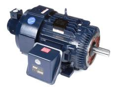
Marathon Blue MAX standard efficiency AC induction motor, highperformance inverter duty, 60hp, 3-phase, 230/460 VAC, 1800rpm, TEBC, NEMA 364TC frame, cast iron, C-face/rigid base mount.
