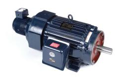
Marathon Blue MAX high efficiency AC induction motor, highperformance inverter duty, 50hp, 3-phase, 230/460 VAC, 1800rpm, TEBC, 326TC frame, cast iron, C-face/rigid base mount.
