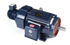
Marathon Blue MAX high efficiency AC induction motor, high-performance inverter duty, 50hp, 3-phase, 230/460 VAC, 1800rpm, TEBC, NEMA 326TC frame, cast iron, C-face/rigid base mount.
