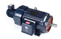
Marathon Blue MAX high efficiency AC induction motor, high-performance inverter duty, 50hp, 3-phase, 230/460 VAC, 1800rpm, TEBC, NEMA 326TC frame, cast iron, C-face/rigid base mount. Dynapar HSD38 encoder included.
