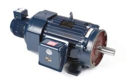
Marathon Blue MAX standard efficiency AC induction motor, high-performance inverter duty, 40hp, 3-phase, 230/460 VAC, 1800rpm, TEBC, NEMA 324TC frame, cast iron, C-face/rigid base mount.
