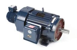
Marathon Blue MAX standard efficiency AC induction motor, high-performance inverter duty, 40hp, 3-phase, 230/460 VAC, 1800rpm, TEBC, NEMA 324TC frame, cast iron, C-face/rigid base mount. Dynapar HSD38 encoder included.
