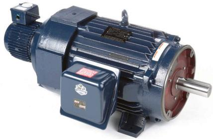
Marathon Blue MAX standard efficiency AC induction motor, high-performance inverter duty, 40hp, 3-phase, 230/460 VAC, 1800rpm, TEBC, NEMA 324TC frame, cast iron, C-face/rigid base mount. Dynapar HSD38 encoder included.
