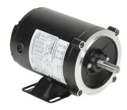
Marathon MicroMAX premium efficiency AC induction motor, high-performance inverter duty, 1/3hp, 3-phase, 230 VAC, 1800rpm, TENV, 56C frame, rolled steel, C-face/rigid base mount.
