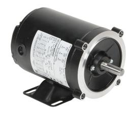
Marathon MicroMAX premium efficiency AC induction motor, high-performance inverter duty, 1/3hp, 3-phase, 230 VAC, 1800rpm, TENV, NEMA 56C frame, rolled steel, C-face/rigid base mount.
