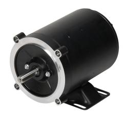
Marathon MicroMAX premium efficiency AC induction motor, high-performance inverter duty, 1/4hp, 3-phase, 230 VAC, 1800rpm, TENV, NEMA 56C frame, rolled steel, C-face/rigid base mount.
