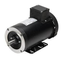
Marathon MicroMAX standard efficiency AC induction motor, high-performance inverter duty, 2hp, 3-phase, 230/460 VAC, 1800rpm, TEFC, NEMA 145TC frame, rolled steel, C-face/removable rigid base mount.
