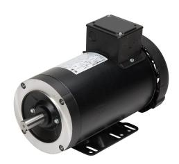
Marathon MicroMAX standard efficiency AC induction motor, high-performance inverter duty, 2hp, 3-phase, 230/460 VAC, 1800rpm, TEFC, 145TC frame, rolled steel, C-face/removable rigid base mount.
