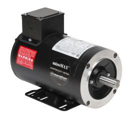
Marathon MicroMAX high efficiency AC induction motor, high-performance inverter duty, 1-1/2hp, 3-phase, 230/460 VAC, 1800rpm, TENV, 145TC frame, rolled steel, C-face/removable rigid base mount.
