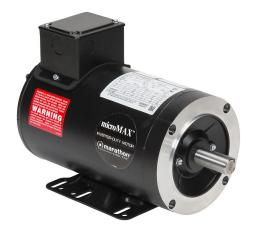
Marathon MicroMAX high efficiency AC induction motor, highperformance inverter duty, 1-1/2hp, 3-phase, 230/460 VAC, 1800rpm, TENV, NEMA 145TC frame, rolled steel, C-face/ removable rigid base mount.
