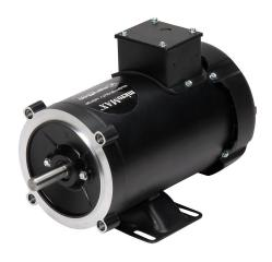
Marathon MicroMAX standard efficiency AC induction motor, high-performance inverter duty, 1hp, 3-phase, 230/460 VAC, 1800rpm, TEFC, NEMA 56C frame, rolled steel, C-face/rigid base mount.
