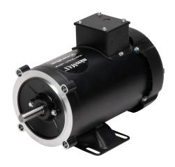
Marathon MicroMAX standard efficiency AC induction motor, high-performance inverter duty, 1hp, 3-phase, 230/460 VAC, 1800rpm, TEFC, 56C frame, rolled steel, C-face/rigid base mount.
