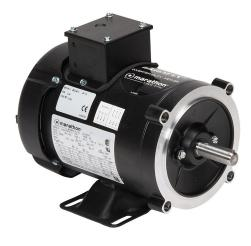
Marathon MicroMAX standard efficiency AC induction motor, high-performance inverter duty, 3/4hp, 3-phase, 230/460 VAC, 1800rpm, TEFC, NEMA 56C frame, rolled steel, C-face/rigid base mount.
