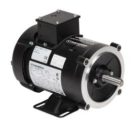
Marathon MicroMAX standard efficiency AC induction motor, high-performance inverter duty, 3/4hp, 3-phase, 230/460 VAC, 1800rpm, TEFC, 56C frame, rolled steel, C-face/rigid base mount.
