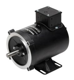
Marathon MicroMAX premium efficiency AC induction motor, high-performance inverter duty, 1/2hp, 3-phase, 230/460 VAC, 1800rpm, TENV, 56C frame, rolled steel, C-face/rigid base mount.
