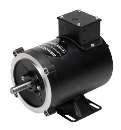
Marathon MicroMAX premium efficiency AC induction motor, high-performance inverter duty, 1/2hp, 3-phase, 230/460 VAC, 1800rpm, TENV, NEMA 56C frame, rolled steel, C-face/rigid base mount.
