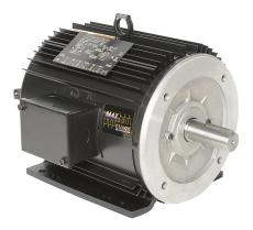
Marathon MAX Plus high efficiency AC induction motor, highperformance inverter duty, 3hp, 3-phase, 230/460 VAC, 1800rpm, TENV, 182TC frame, aluminum, C-face/rigid base mount. Dynapar HS20 encoder included.
