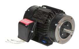
Marathon MAX Plus high efficiency AC induction motor, high-performance inverter duty, 2hp, 3-phase, 230/460 VAC, 1800rpm, TENV, 145C frame, cast iron, C-face/removable rigid base mount. Dynapar HS20 encoder included.
