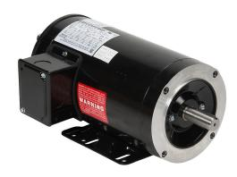
Marathon MAX Plus high efficiency AC induction motor, high-performance inverter duty, 1-1/2hp, 3-phase, 230/460 VAC, 1800rpm, TENV, 145TC frame, rolled steel, C-face/removable rigid base mount. Dynapar HS20 encoder included.
