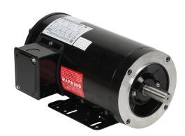
Marathon MAX Plus high efficiency AC induction motor, highperformance inverter duty, 1-1/2hp, 3-phase, 230/460 VAC, 1800rpm, TENV, NEMA 145TC frame, rolled steel, C-face/ removable rigid base mount. Dynapar HS20 encoder included.
