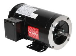
Marathon MAX Plus high efficiency AC induction motor, highperformance inverter duty, 1hp, 3-phase, 230/460 VAC, 1800rpm, TENV, 56C frame, rolled steel, C-face/removable rigid base mount. Dynapar HS20 encoder included.
