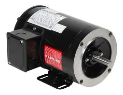
Marathon MAX Plus premium efficiency AC induction motor, highperformance inverter duty, 3/4hp, 3-phase, 230/460 VAC, 1800rpm, TENV, NEMA 56C frame, rolled steel, C-face/removable rigid base mount. Dynapar HS20 encoder included.
