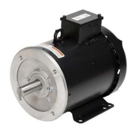
Marathon MicroMAX high efficiency AC induction motor, highperformance inverter duty, 3hp, 3-phase, 230/460 VAC, 1800rpm, TEFC, 182TC frame, rolled steel, C-face/removable rigid base mount.
