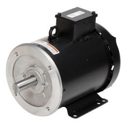
Marathon MicroMAX high efficiency AC induction motor, highperformance inverter duty, 3hp, 3-phase, 230/460 VAC, 1800rpm, TEFC, NEMA 182TC frame, rolled steel, C-face/removable rigid base mount.
