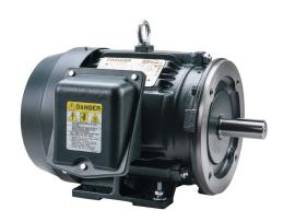
Toshiba SD premium efficiency AC induction motor, high-performance inverter duty and severe duty, 1-1/2hp, 3-phase, 230/460 VAC, 1200rpm, TEFC, 182TC frame, cast iron, C-face/rigid base mount.
