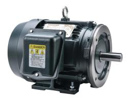
Toshiba SD premium efficiency AC induction motor, highperformance inverter duty and severe duty, 1-1/2hp, 3-phase, 230/460 VAC, 1200rpm, TEFC, NEMA 182TC frame, cast iron, Cface/rigid base mount.
