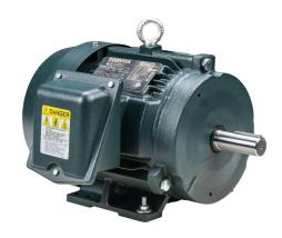
Toshiba SD premium efficiency AC induction motor, high-performance inverter duty and severe duty, 1-1/2hp, 3-phase, 230/460 VAC, 1200rpm, TEFC, NEMA 182T frame, cast iron, rigid base mount.
