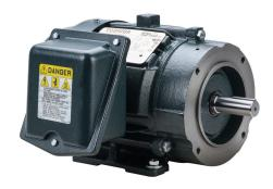
Toshiba SD premium efficiency AC induction motor, high-performance inverter duty and severe duty, 1-1/2hp, 3-phase, 230/460 VAC, 1800rpm, TEFC, NEMA 145TC frame, cast iron, C-face/rigid base mount.
