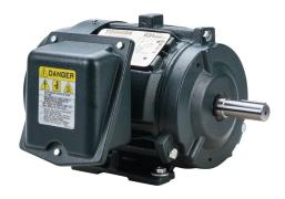
Toshiba SD premium efficiency AC induction motor, high-performance inverter duty and severe duty, 1-1/2hp, 3-phase, 230/460 VAC, 1800rpm, TEFC, NEMA 145T frame, cast iron, rigid base mount.
