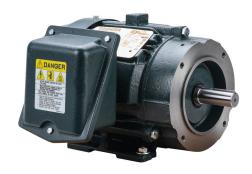
Toshiba SD premium efficiency AC induction motor, high-performance inverter duty and severe duty, 1-1/2hp, 3-phase, 230/460 VAC, 3600rpm, TEFC, NEMA 143TC frame, cast iron, C-face/rigid base mount.
