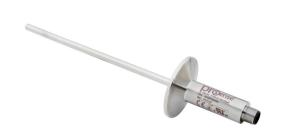
ProSense temperature transmitter, integral Pt100 RTD, 0 to 300 deg F, 6mm probe diameter, 150mm insertion length, 1-1/2in sanitary tri-clamp process connection, 4-20 mA analog output, 4-pin M12 quick-disconnect.
