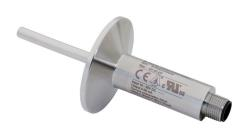
ProSense temperature transmitter, integral Pt100 RTD, 0 to 300 deg F, 6mm probe diameter, 50mm insertion length, 1-1/2in sanitary tri-clamp process connection, 4-20 mA analog output, 4-pin M12 quick-disconnect.
