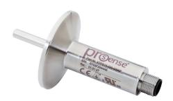
ProSense temperature transmitter, integral Pt100 RTD, 0 to 300 deg F, 6mm probe diameter, 30mm insertion length, 1-1/2in sanitary tri-clamp process connection, 4-20 mA analog output, 4-pin M12 quick-disconnect.
