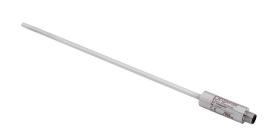
ProSense temperature transmitter, integral Pt100 RTD, -40 to 140 deg F, 6mm probe diameter, 260mm insertion length, 4-20 mA analog output, 4-pin M12 quick-disconnect.
