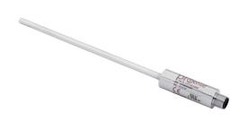
ProSense temperature transmitter, integral Pt100 RTD, 0 to 300 deg F, 6mm probe diameter, 160mm insertion length, 4-20 mA analog output, 4-pin M12 quick-disconnect.
