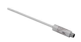
ProSense temperature transmitter, integral Pt100 RTD, 0 to 100 deg C, 6mm probe diameter, 160mm insertion length, 4-20 mA analog output, 4-pin M12 quick-disconnect.
