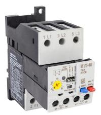
Eaton XT series electronic overload relay, 0.33-1.65A adjustable, solid state, ground fault protection, stand-alone power connection(s), DIN rail or panel mount. For use with any contactor.
